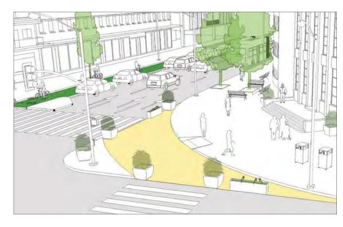
Reduces the time pedestrians interact with vehicles and allows for a single crossing point where there may have been three separate crossings
