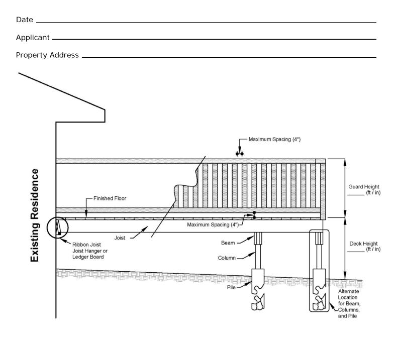
**NOTE:** This shows a typical deck. You may need to draw a separate elevation if this does not represent your proposed deck
