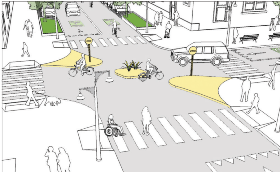
Figure 5.15: Diverter (Source: NACTO Global Street Design Guide)
