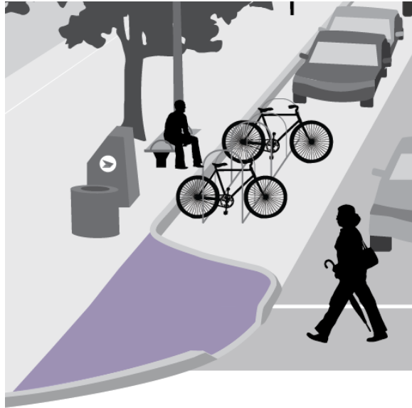
Figure 5.9: Curb Extension on an Arterial Street
