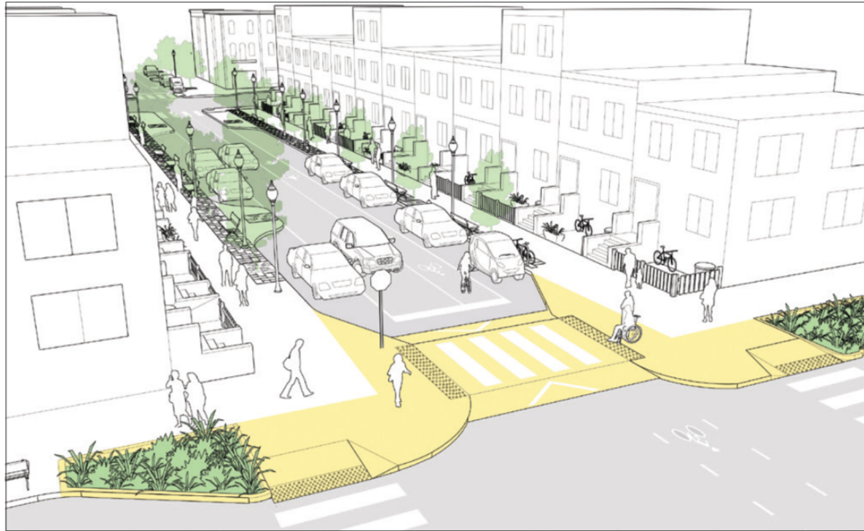
Figure 5.16: Raised Crossing (Source: NACTO Global Street Design Guide)
