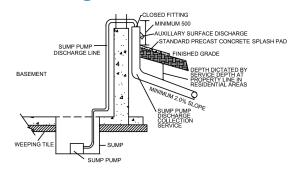
Roof leaders (downspouts) or any other storm water source cannot be connected to the sump pump discharge collection service line.
