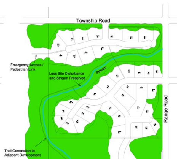
Figure 15: Example of a quarter section that has developed according to Conservation Design principles. Note: the minimal amount of site disturbance and the conservation of the stream and wildlife corridor.
